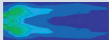
Cold air distribution without guide vane
