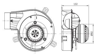
for solid fuel heating systems, single inlet, Ø 150
