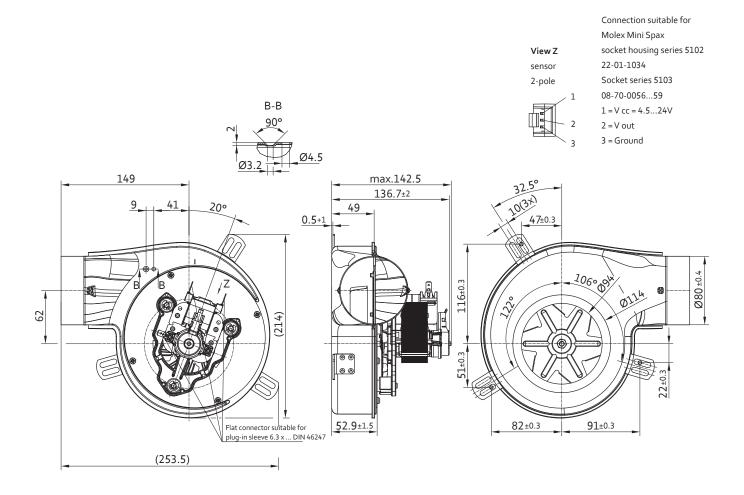
for solid fuel heating systems, single inlet, Ø 180
