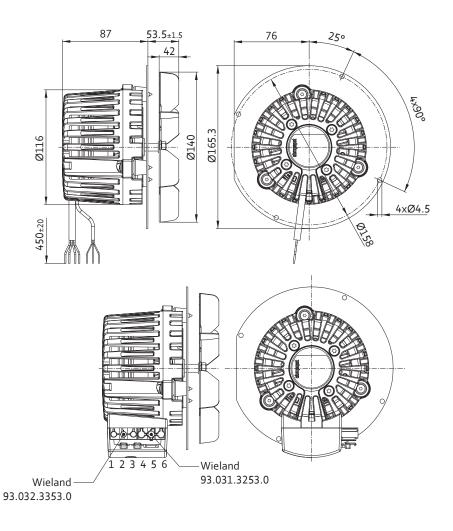
for solid fuel heating systems, single inlet, Ø 150
